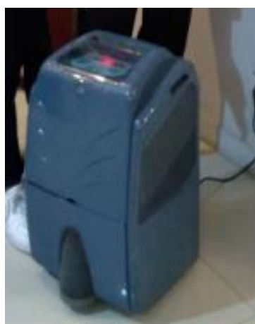
Figure 4 Dehumidifier as a room humidity regulator.
