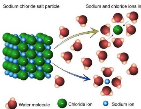
Figure 1 The dissociation of salt to form chloride and sodium ions. Source: Crundwell (2019)
