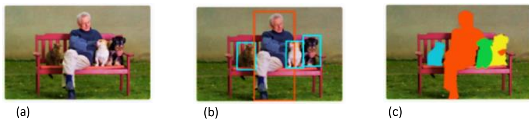
Figure 11 (a) Object classification, (b) Object detection, and (c) Object segmentation (O’Shea, & Nash, 2015).
